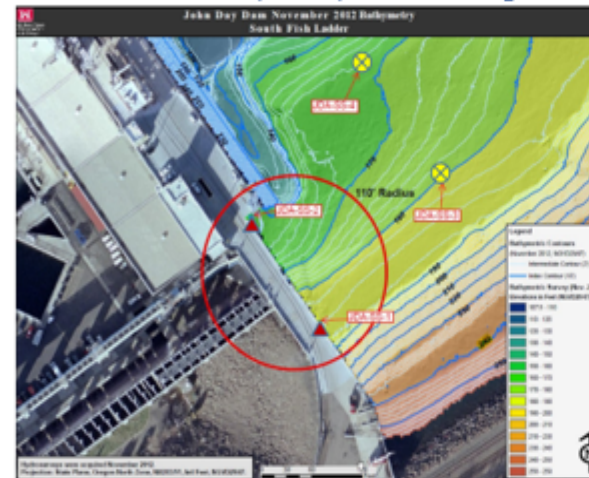
Figure 4-1. The John Day South Fish Ladder Exit and Locations of the Four Temperature Profile Strings; JDA-SS-1 and JDA-SS-2 (red triangle) are attached to the Structure, while JDA-SS-3 and JDA-SS-4 are Floating Strings (yellow circle).
